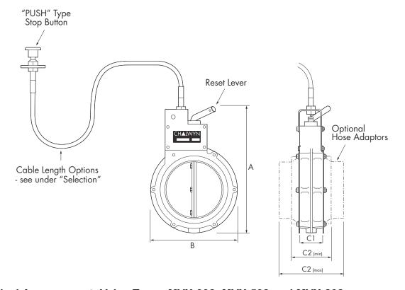
Typical Arrangement: Valve Types MVX-302, MVX-502 and MVX-802
